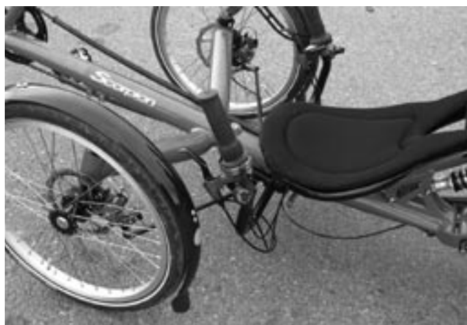
Note disc brakes and true quick-release front axles. Also, the seat is a BodyLink shells seat with optional Airflow cushion.
