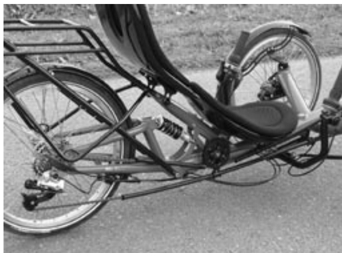
The Scorpion has a rear suspension, an optional V-parking brake and super-tough (and expensive) rear rack.
