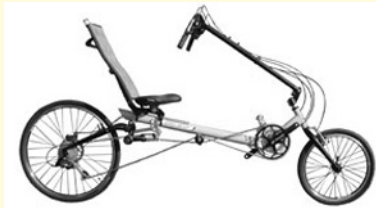
The 2006 Burley Spider with its unique rear suspension and new Fox shock, see page 16
