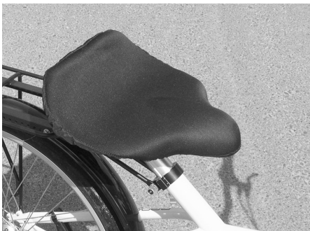
The Fusion seat; note reclined seat post
