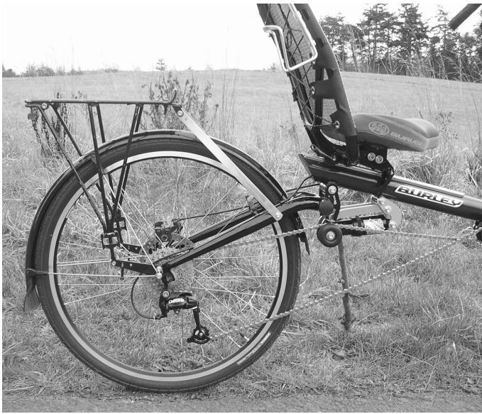
The Spider's unique suspension system. Note seat base angle (most upright position)
