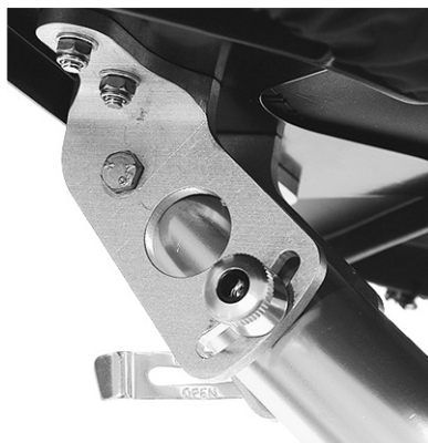
The RANS Fusion seat quick-release controls the angle of the seat base on the seat post
