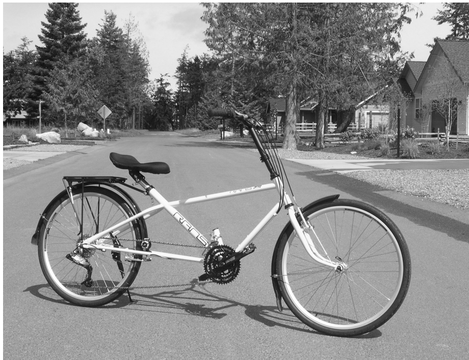
Our 2005 test bike with unavailable tall stem and 2005 2.5" rise bars
