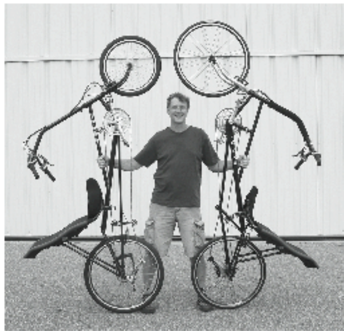
Above: RANS' Randy Schlitter shows the 2006 RANS Stratus XP with dual 26" wheels (right) alongside the stock 2005 26"/20" model (left). The Stratus XP will be available by the time you read this. Right: The Stratus XP chopper bars
