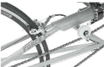
The F5's trussed (triangulated) frame
