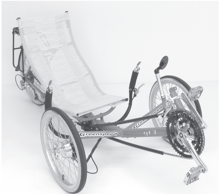
At first glance the GT-3 make look like your average Greenspeed trike. However, it has 16" wheels (vs. a GTO's 20" wheels) and the width is 2.5" narrower than the GTO, which makes it easier to get it through door — and it folds.
