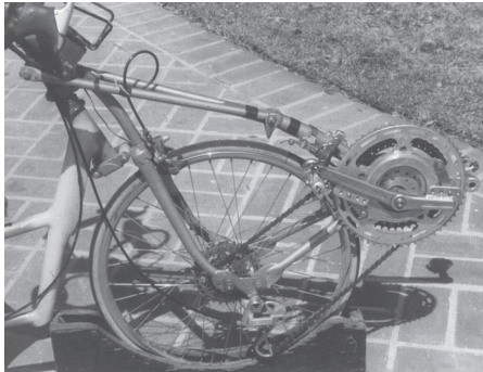
View of early tube-frame FWD recumbent with my version of the "Rotor Crank"
