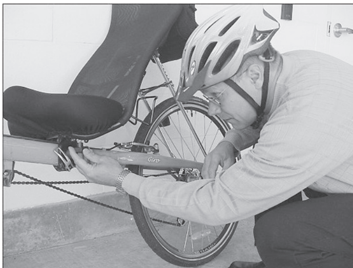
Two large plastic wing nuts with metal inserts which I purchased at a local hardware store hold the seat to the new seat frame brace. No tools needed to remove or install the seat now.
