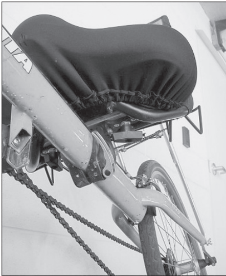
This photo shows both the large plastic wing nuts under the seat and the smaller wing nuts to hold the rear seat brackets to the frame near the rear drop outs.
