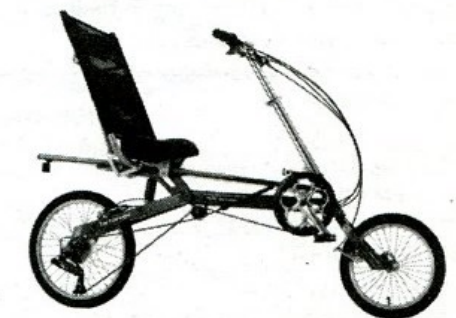
Left: The folding Tartaruga is an interesting EZB/CLWB design that is not available in North America as of yet.
