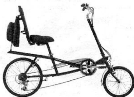
While it doesn't have trendy styling or wide range gearing, the entry level KHS RC 1620 recumbent has a full CroMo frame and fork
