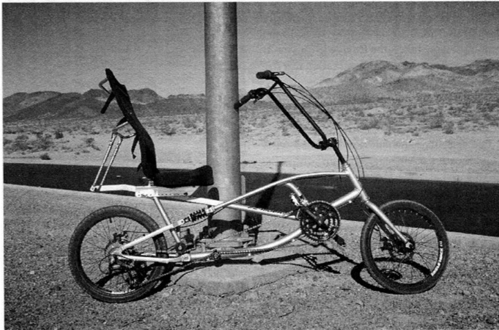
Sun's EZ Rider rear suspension LWB comes in HiTen, CroMo and alum. (John Riley)
