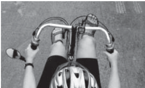
Bacchetta Ergonomics 101: the "tweener" bars. The TerraCycle Glide Flex stem allows the Bacchetta riser to recline. Optimum ergonomics on a Giro, Strada or Corsa require that your knees just clear the bars during the pedal stroke. The system is unique and works very well. (Photo courtesy of Shari Bernhard)
