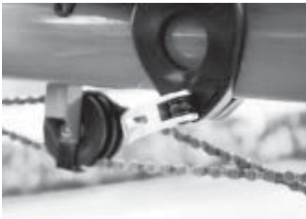
Bacchetta's X-path idler and seat adjuster
