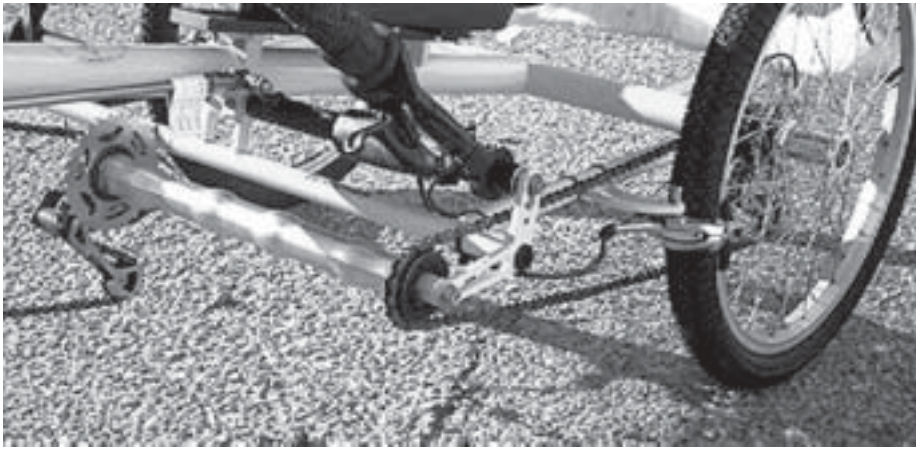
Note Penninger jackshaft and two rear derailleurs
