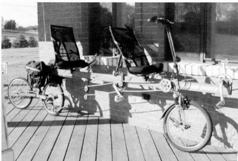
The Cubed Deuce, our inline trike tandem. Yes, that's a lot of chain! Runs quiet and shifts great—D.M. Fulks
