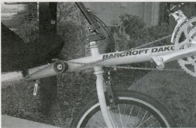
RIGHT: Author Paul Kern and his Barcroft. LEFT: Note the Barcrofts X-path chain idler, RANS seat and Flip It stem/riser
