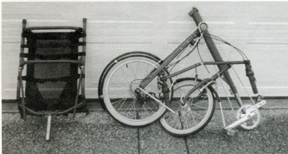
The Phaser folded with seat removed. This can be done in less than one minute. Note the seat post. The post fits into the head tube at the end of the mainframe/boom and then into the swing arm where it locks the frame sections into place. The bike will not fold until the seat post is removed.
