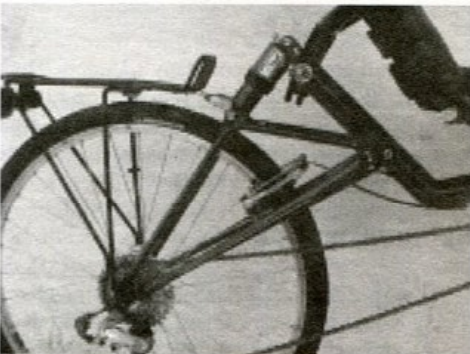
Vision's new triangulated swing arm and air shock location. This design is said to require significantly less shock pressure than previous designs.
