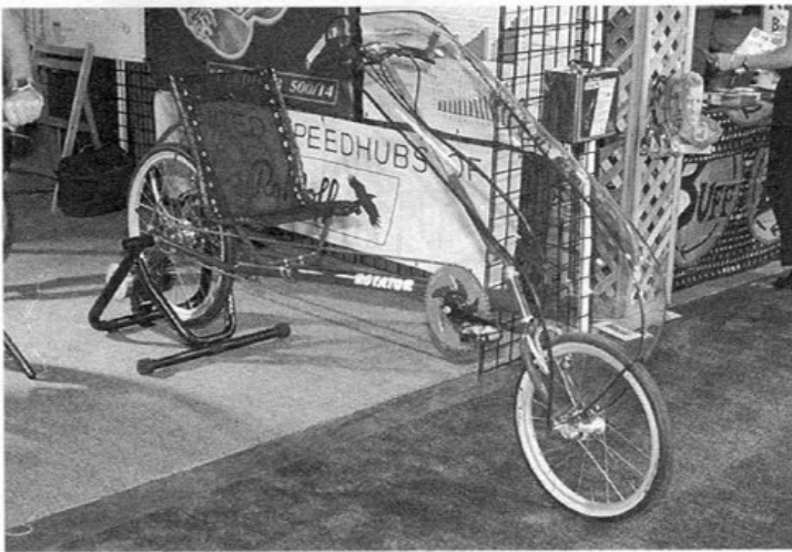
A one-off Rotator with Rohloff hub and 26-inch drive wheel at Rohloff booth—John Riley
