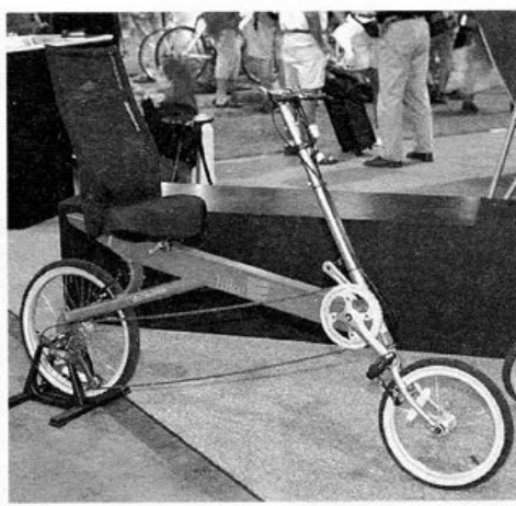
The 2001 BikeE CT is now $550. Note welded on rear stays, bigger seat base and the CT is now powdercoated instead of anodized—John Riley
