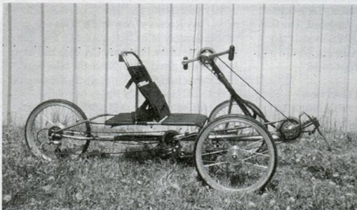
The Angletech Quadraped hand/foot power trike. A similar foot crank only version is the TriSpeeder
