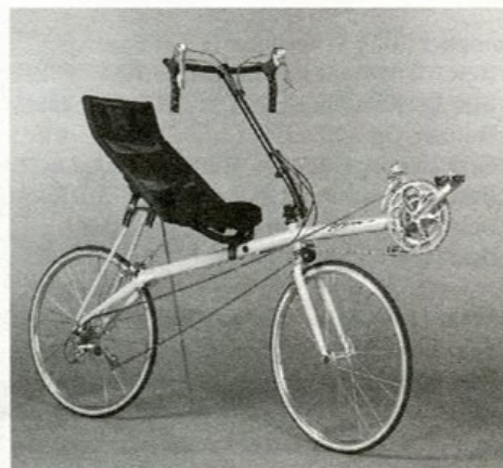
The Vision Saber with dual 24-inch wheels photo courtesy of Vision
