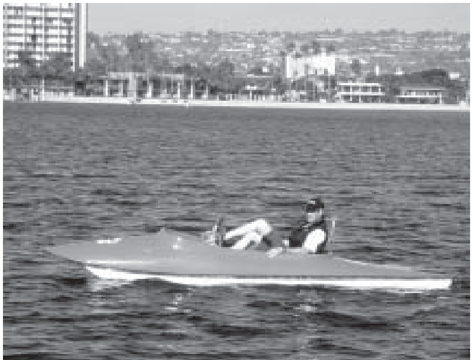
John Howard's Wave Walker. This is certainly the most high performance looking HPB. It is a catamaran design (with a tunnel hull), though it is actually more narrow than it looks in this picture. Note the rather aggressive high pedal/BB position. We were not able to see or ride this HPB, though would love too.
