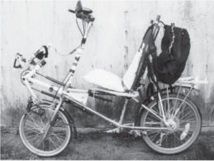
Ming Dinh's BMX "shopper." Note the bolt-on boom utilizing a road fork, frame tube and a clamp bolted to a wood wedge in the frame—Ming Dinh
