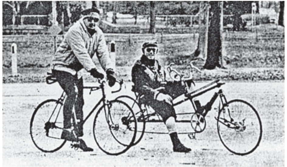
Dan Henry and wedgie rider chat. Note dual suspension and remote above-seat steering—photo circa 1968
