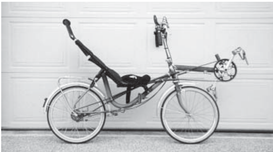
Tony's dual 20" folder with Nexus 7 hub and Vision seat—RCN
