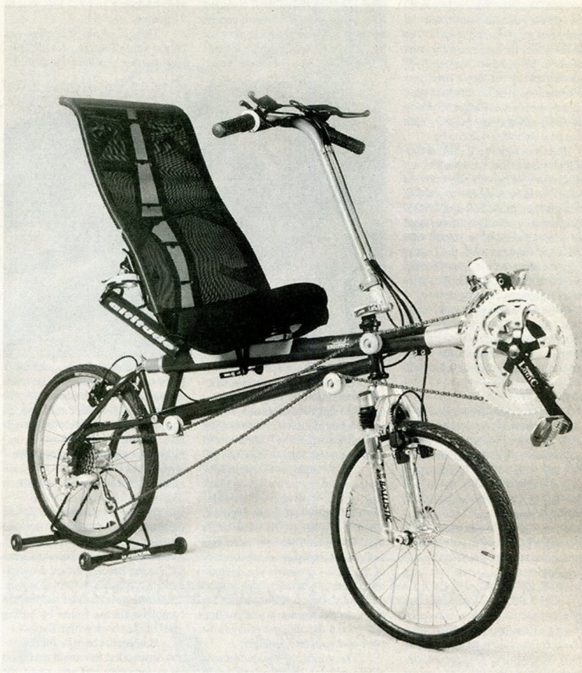
The Angletech Altitude now has a lower tail tube, curved and painted boom and a new one-idler chain management system—Angletech
