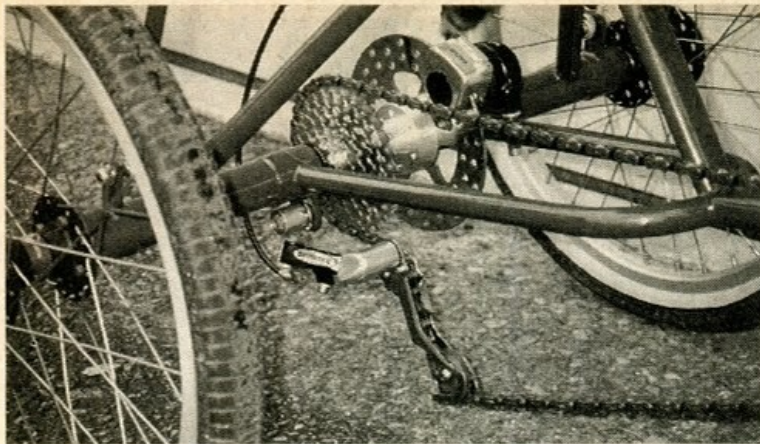
The Tritan's rear end seems complex but is actually quite simple. The Sachs brake is very strong. Just the right rear wheel is driven and braked, the left rear wheel has a separate axle.
