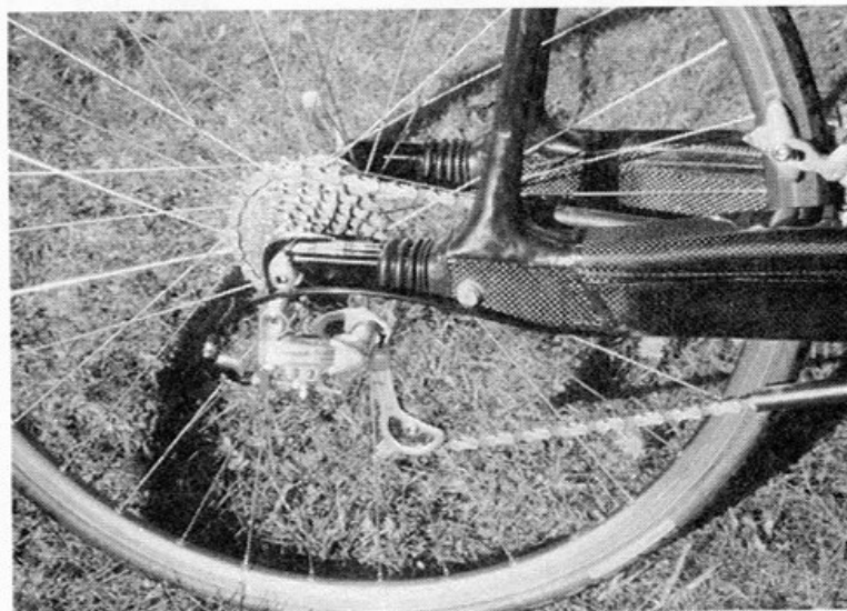
Note rear suspension in the dropouts—Jim Langley
