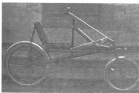
This is Henri's second Velocar. It has a direct chain drive and larger rear wheel, and was a higher off the ground. Photo courtesy of Henri Chais
