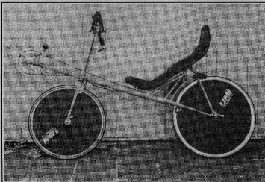
"M5 with suspension with a 28" rear wheel and your choice of 24", 26", or 28" front wheels" (Photo by Bram Moens)
